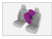
Driver's seat has a far side airbag in addition to the side airbag. Location of far side airbag is shown in the
